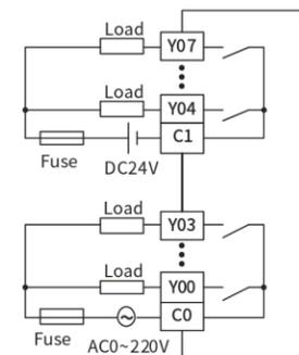
Figure 11 Relay output equivalent circuit
