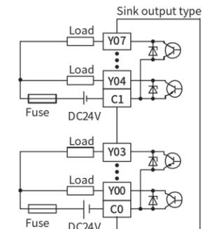
Figure 12 Transistor output equivalent circuit
