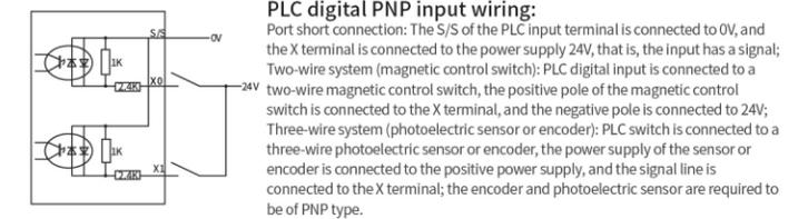
Figure 10 Input wiring diagram
