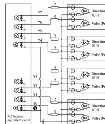
Figure 13 Pulse output wiring diagram
