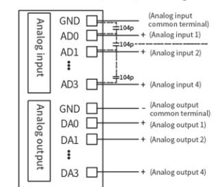
If the analog input is unstable, please add 104p ceramic capacitor or external magnetic ring filter as appropriate to increase the anti-interference ability
